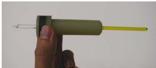
FIG. 5. Picture of a typical NMR sample in a spinner.
