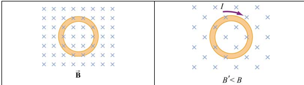
Figure 10.1.3 Inducing emf by varying the magnetic field strength
