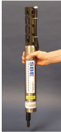
Figure 3: A typical vehicle CTD: the Sea-Bird SBE49 [3]
