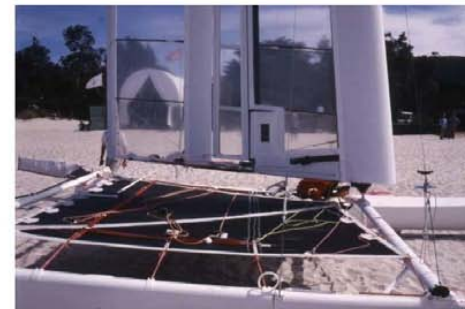
Figure 16: Three element wing sails have been found to be more efficient than two element sails in the C-Class catamaran.
