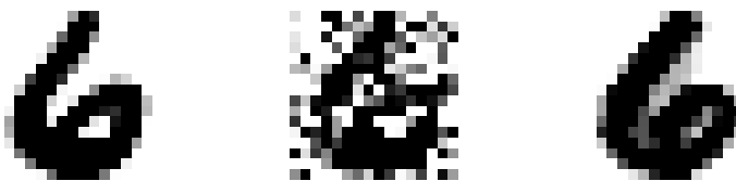
Figure 2.1. Reconstruction of the digit “6”: Original (left), Noisy (middle) and Reconstruction (right). Here n = 16 \times 16 = 256 pixels. Source [RT11].
