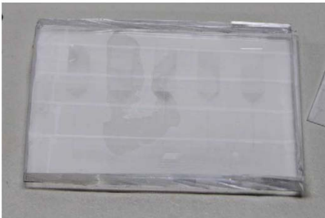
Device Partially Bonded To Glass
