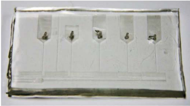
Freshly Bonded PDMS Device
