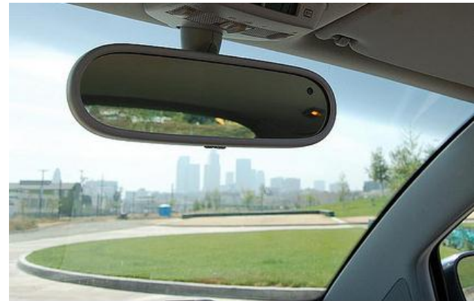
A rear view mirror with an electrochromic layer for dimming during night time use
