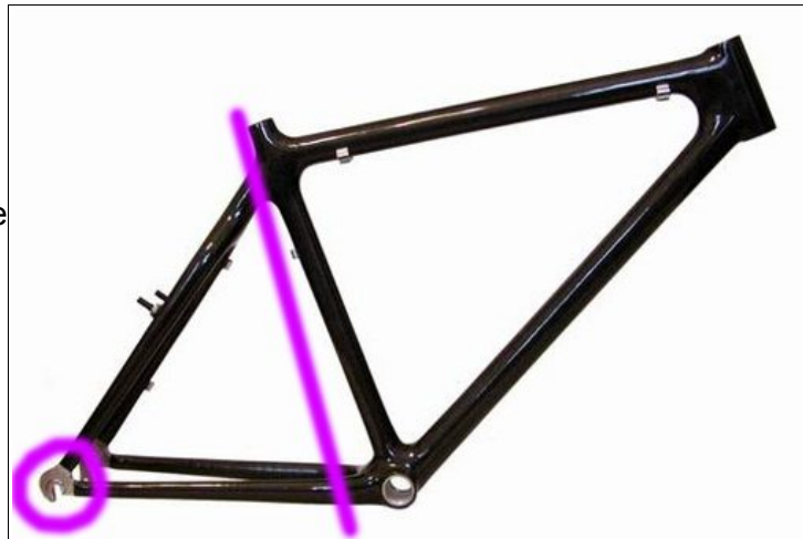
Illustration 22: Cut on the line and leave a bit of material on the bottom of the frame, behind the bottom bracket, so that there is ample material remaining to weld the stand to. Image Credit: Jarrett, 2010.
