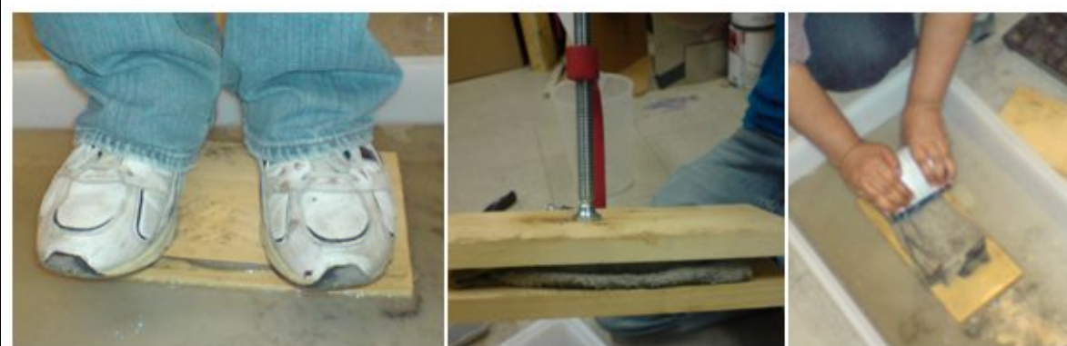
Illustration 15: Different methods tested for de-watering. Vertical pressing via weight (right), vertical pressing via clamp (middle), and pressing with roller (left). Image Credit: Moncivaiz and Hasan 2010
