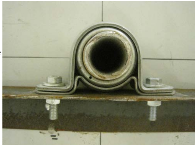
Illustration 21: The sleeve that holds the inner drums axle. Image credit: Lu, 2010.
