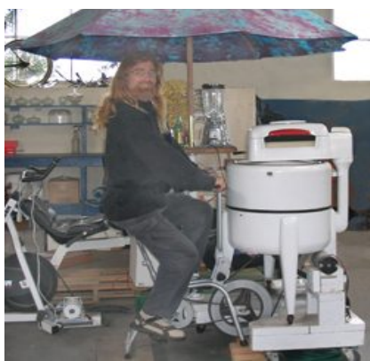
Illustration 1: Household electric washing machine converted to pedal power (via exercise bike.)
