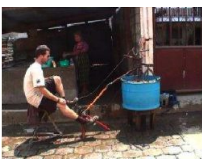
Illustration 3: Vertical-axis bicilavadora built by Maya Pedal. Image Credit: Raduta, 2005.
