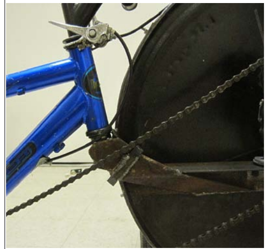
Illustration 24: Close-up of the bike to drum connection. Photo Credit: Lu 2010.
