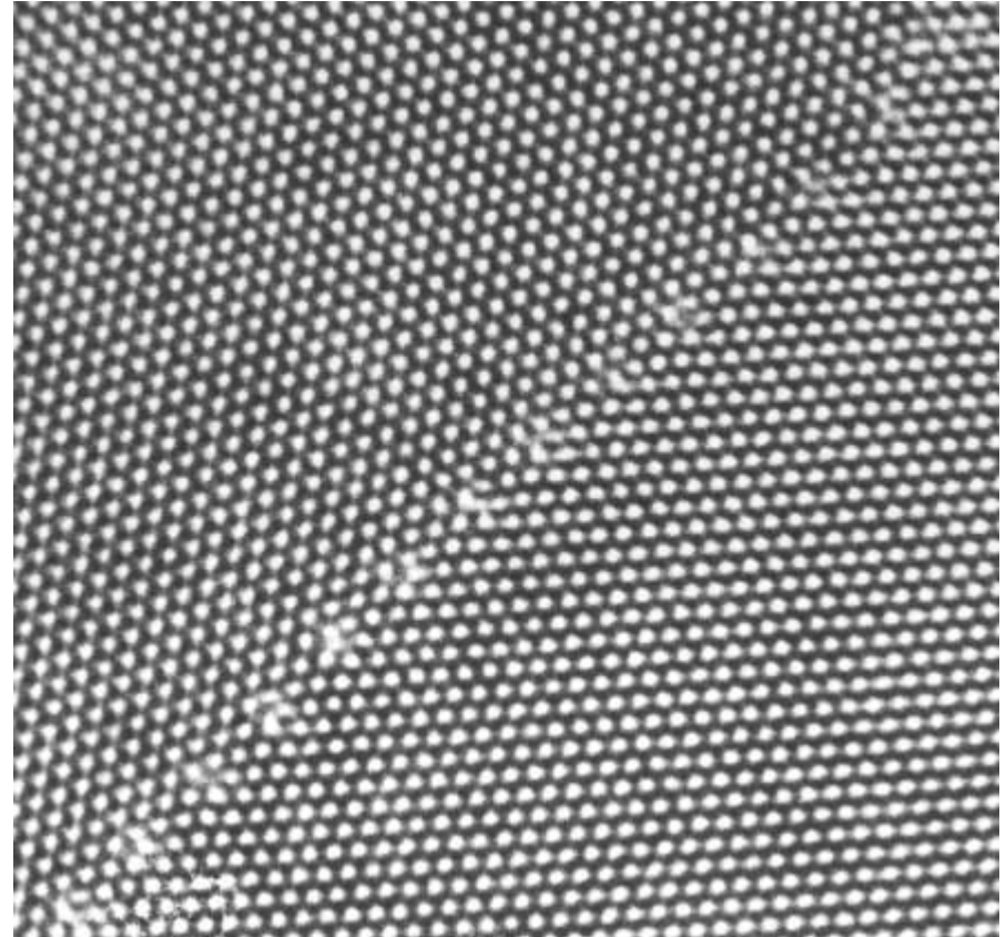
TEM image of a grain boundary in pure Al
